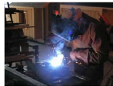
Cory welding the front frame
